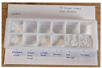
Polystyrene balls and marbles give the largest measurable difference between the amount of ground material produces and how visually coarse/fine the material is.
